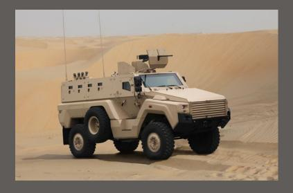
KAYA is specially designed and developed as a Mine Resistant Ambush Protected Personnel Carrier based on torsionally flexible chassis. KAYA provides enhanced mine and ballistic protection along with superior mobility in a wide range of demanding terrains under diverse climatic conditions. Single cabin monocoque body of KAYA carries up to ten troops including the driver and commander.
