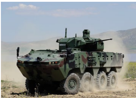
PERSONNEL CARRIER WITH MIZRAK 30 MM MEDIUM CALIBER REMOTE CONTROLLED TURRET
